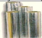
Fujairah Rockwool Preformed Pipe Section faced with reinforced aluminium foil conforming to ASTM C-547 and equivalent BS 3958-4 is intended for the thermo-acoustic insulation and fire protection of pipe works operating at high temperatures. The pipe insulation is manufactured from long non-combustible rock fibers with a high performance binder. It is easy to cut, fit, handle and has high levels of thermal efficiency and strength. Each section is split and hinged for easy, snap-on applications.
